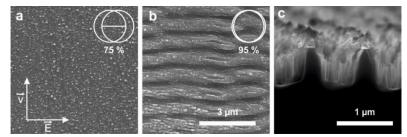
Fig. 1. SEM images of a laser-structured surface: a) 75 % pulse overlap, b) 95 % pulse overlap, c) cross-section image of etched structures in silicon. v and E vectors show scanning direction and electric field polarisation respectively.
