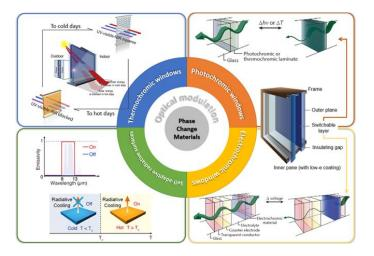
Figure 1. Schematics of adaptive for optical modulations, their mechanisms, and applications in energy-efficient windows: thermochromic windows, photochromic, electrochromic and self-adaptive radiative surfaces. Electrochromic and photochromic SW colour in response to the applied voltage and light, respectively. Thermochromic SW responses to the temperature.
